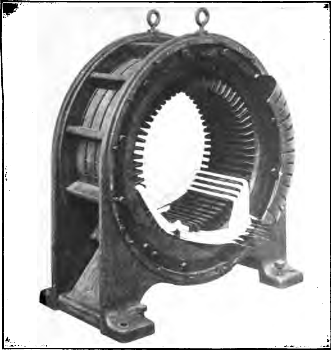
FIG. 97.—Windings partially assembled in a 25-cycle synchronous motor.
